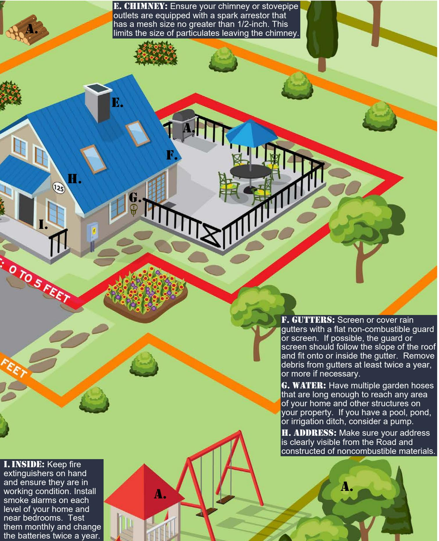
**F. GUTTERS:** Screen or cover rain gutters with a flat non-combustible guard or screen. If possible, the guard or screen should follow the slope of the roof and fit onto or inside the gutter. Remove debris from gutters at least twice a year, or more if necessary.
